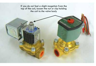
If the coil is good you probably have a bad diaphragm, stuck plunger, or a piece of debris holding the valve open. A small speck of sand in the right place on the valve seat is all it takes to keep the valve from closing properly.
